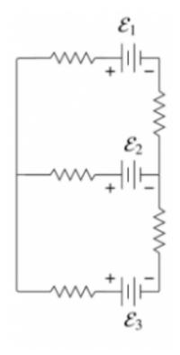
**G52.** The diagram below shows a schematic design of a circuit with 3 resistors and 3 EMFs. The EMFs are  $?_1 = 15.0 \text{ V}$ ,  $?_2 = 10.0 \text{ V}$ , and  $?_3 = 18.0 \text{ V}$ . The resistors have  $R_1 = 3.00 \Omega$ ,  $R_2 = 2.00$ , and  $R_3 = 1.00 \Omega$ . Find the current through  $R_2$  and its direction.
