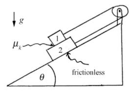
**B61**. Masses 1 and 2 are connected as shown in a ramp/pulley system on planet 3TTE (g = 8.3). The left block (m<sub>1</sub>) has a weight of 249 N, while the right block (m<sub>2</sub>) has a weight of 166 N. Angle theta is 60 degrees. If the coefficient of static friction is 0.55 and kinetic friction is 0.45, what is the acceleration of the system?
