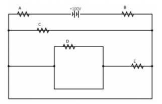
**G70.** Where (A, B, and C) is the current largest in the following circuit? All resistors are identical.
