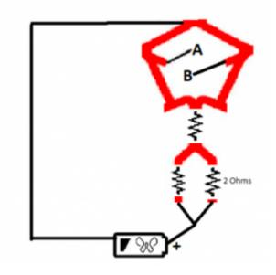
**G63.** Find the equivalent resistance between the terminals A and B in the network shown below.
