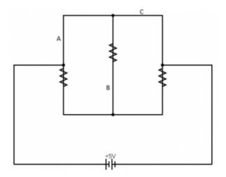
**G71.** In the diagram below, what is the equivalent resistance between point A and point B? Calculate the current in each resistor if a potential difference of V = 100 V is applied between points A and B.
