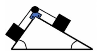
**B56**. If m = 20 kg, M = 13 kg,  $\theta$ = 25°, µs=0.25, µk = 0.20, find the acceleration of the blocks when they are released.
