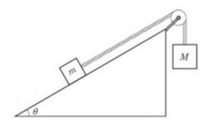
**B62**. A mass of 3 kg sits on an inclined plane, making an angle of 20° with the horizontal. A rope is attached to mass and placed over a pulley at the top of the incline, with a 1 kg mass attached to the other end of the rope. If  $\mu$ k = 0.33, what is the acceleration of the system?
