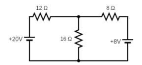
**G41.** Find the equivalent resistance in the circuit below.
