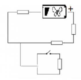
**G65.** If you place a voltmeter in parallel with a  $5.0-\Omega$  resistor, only 5% of the main current passes through it. Compute the resistance of the voltmeter and the current passing through the 15.0-V EMF source.
