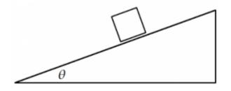
**B48**. A force,  $F_1$ , can be used to move a block up and inclined plane at a constant velocity. Another force,  $F_2$ , can be used to move the block down the same incline. Find the coefficient of kinetic friction between the box and the inclined plane given that you know  $F_1 = 10F_2$  and the forces are applied as shown in the figure. The angle, alpha, between the incline and the plane is 15 degrees.
