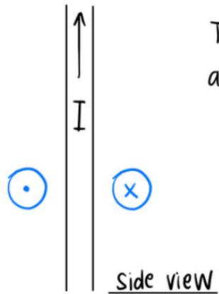
The magnetic field lines form concentric circles around the straight, current-carrying wire.
