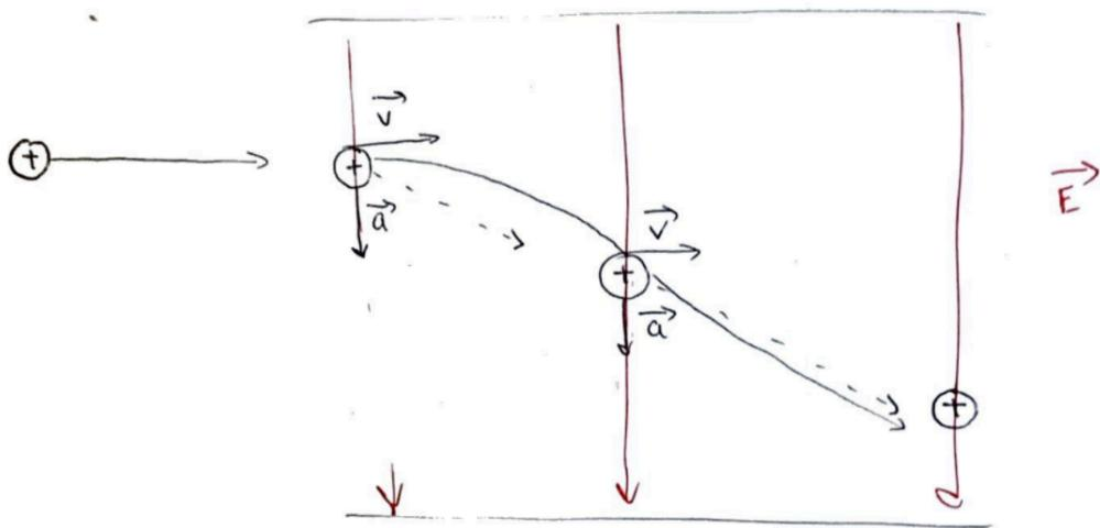
$\vec{E}$  adds vertical component (accelerative force) to initial horizontal velocity, causing parabolic movement (just like gravity on a horizontally launched projectile)
