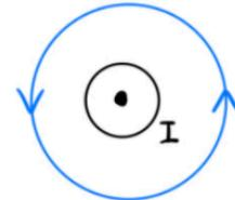
The right hand rule indicates the magnetic field lines are directed counter clockwise when assessing the wire from a top view.
