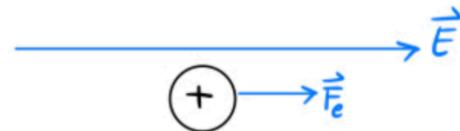
The force exerted on a positively-charged particle by an electric field will act in the same direction as the electric field.
