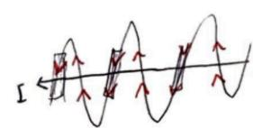
$\vec{B}$  is pointing down behind the coil, up in front (do RHR with your thumb pointing left; fingers curl in direction of  $\vec{B}$ )
