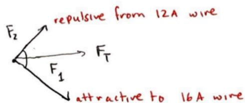
$$\frac{F_1}{l} = \frac{\mu_0 (6\text{ A})(12\text{ A})}{2\pi (0.08\text{ m})} = 0.00024 \frac{\text{N}}{\text{m}}$$
