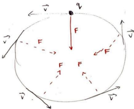
Using RHR at any point in the circle (with corresponding tangential velocity & inwardly directed  $\vec{F}$ ), the  $\vec{B}$  must be going into the page relative to the proton's plane of travel.
