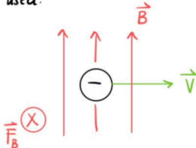
The force exerted on a negatively-charged particle by a magnetic field will act perpendicular to both  $\vec{v}$  and  $\vec{B}$ . The right hand rule will indicate a direction directly opposite to the direction  $\vec{F}_B$  acts on.
