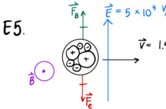
① The force exerted on the negative particle by the **electric field** is opposite in direction to the electric field itself.
