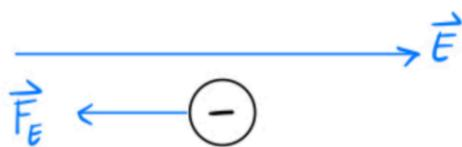
The force exerted on a negatively-charged particle by an electric field will act in the opposite direction as the electric field.
