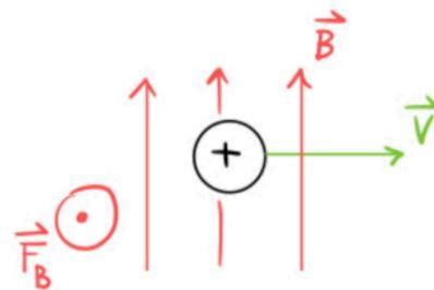
The force exerted on a positively-charged particle by a magnetic field will act perpendicular to both  $\vec{v}$  and  $\vec{B}$ . The right hand rule can be used.
