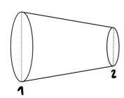
flow rate =  $A \cdot V$ Rinciple of continuorly  $A_1V_1 = A_2V_2$
