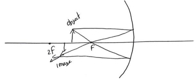
The above situation shows how a concare mirror with an object placed between the focal point and centre of curvature can produce a real and inverted image
