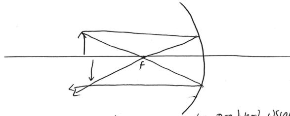
A real and inverted image can be produced using a concave mirror, when the object is placed outside of the focal Point.
